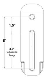
\* Elongated slotted hole to accomodate most existing pole drill patterns.
