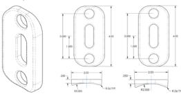
**ROUND POLE ADAPTER (RPA)** – When using round poles, specify Round Pole Adapter (RPA). Specify RPA4 when installing on 3"-4" round poles, and RPA5 when installing on 5"-6" round poles.
