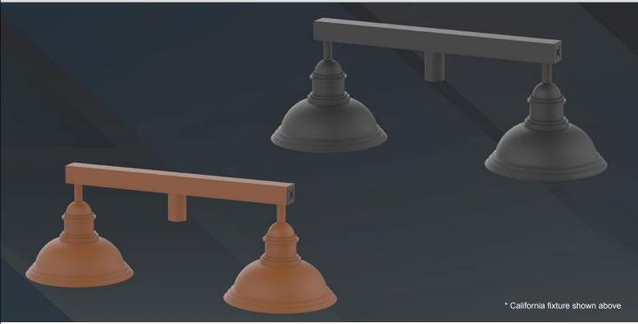
Inline Cross Pendant Arms are constructed of square steel tubing (11G) and can mount up to 5" diameter of Pole or Tenon. The arms are secured with 3/8" stainless steel Allen Sets Screws
