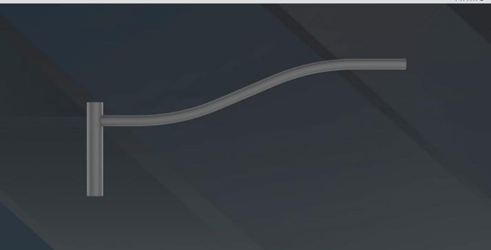
Architectural Arm 16 is constructed of extruded aluminum tubing. This mast arm integrates with poles or tenons of 3-1/2", 4", 4-1/2", or 5" OD and is secured with 3/8" stainless steel Allen set screws.
