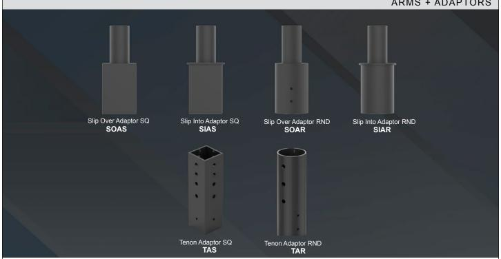
Our Adaptors are constructed of square or round steel tubing (11G) with a 2-3/8" OD tenon. Each adaptor is secured with 3/8" stainless steel Allen Set Screws and use black plastic snap-in
